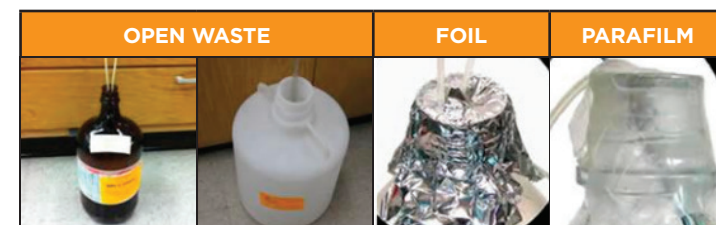
FIGURE 11.5A – Improper LC Waste Collection Processes
